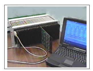
High-Voltage PIN diode drivers can be configured as PC-controllable cards that are compatible with standard 19 inch rack mounting. On-board self test of temperature, currents, voltages, and logic states assures reliability. Control and self-test functions are transmitted by a built-in optically-isolated 9-pin serial port.
