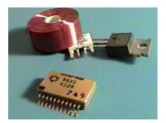
YIG drivers accept a voltage input or a binary word and output a stable, low-noise current for driving the tuning coil of typical YIG tuned devices. Units can be customized to suit particular requirements and specifications. Internal linearizers, sense resistors, and high speed FM or dithering outputs are available.
