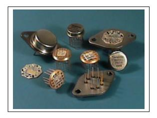
Direct drop-in replacements are available for many hard-to-find components. Commercial and full MIL-Spec devices can be provided. Costly and impractical redesign of systems can be avoided by extending the life of these legacy parts. TO – packages, flatpacks and DIP devices are among the many styles offered.
