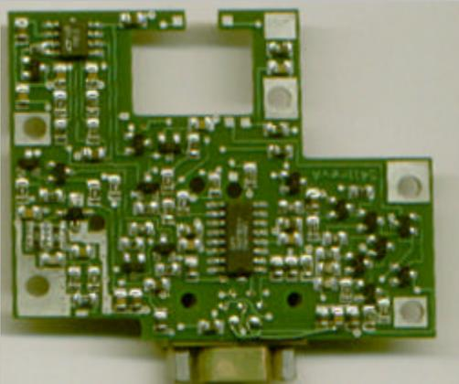
Multi-function drop-in subassembly with RF amplification, high-speed video pulse detection, and several PIN switch driver circuits in a user-friendly shaped layout. Backside is fully grounded for low loss and low-noise operation.
