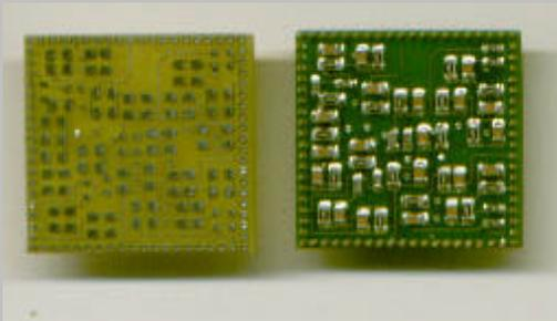
BGA footprint 5 channel, 10 output +250V PIN diode driver. Constructed with brass contact feet and high-temp solder to enable use as a BGA daughter board. Dual-sided assembly with airborne avionics compliant layout.
