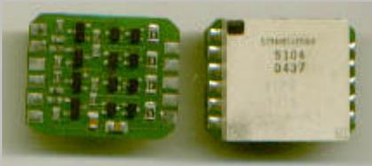
Small 4 channel PIN driver. Chamfered corners allowed this design to maximize use of available floor space within the housing.
