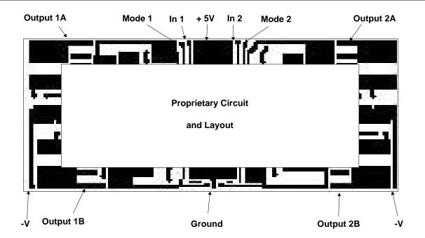
Two Channel High Speed X-Nor PIN Driver, Dual Outputs
