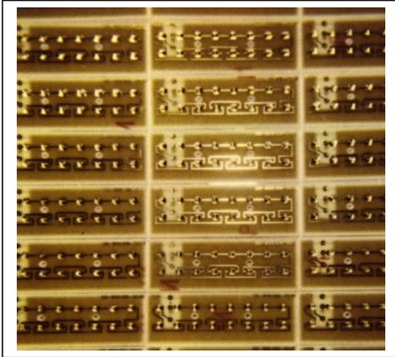
Chip-On-Board (COB) is a form of direct die attach which minimizes cost and size in many applications. The unpackaged dice are mounted onto a prepared PC board, wirebonded, and coated for protection. COB can also be used in conjunction with standard SMT devices.
