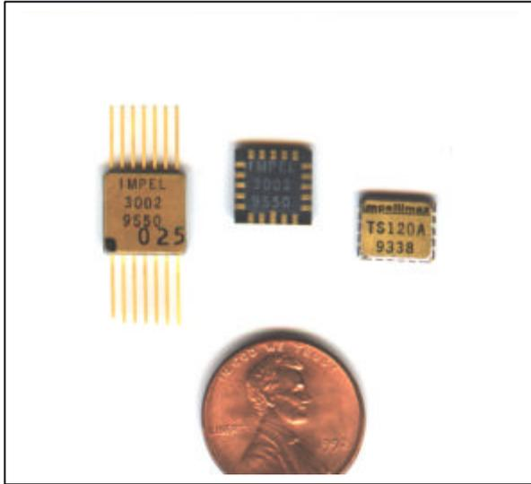
Hybrid Tilt Sensor Pre-amplifiers generate AC bias for electrolytic tilt sensors and produce a DC output current which is a function of the tilt of the device. They require only a single power supply, which can vary over a wide range of voltage.
