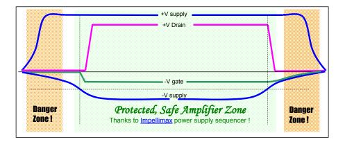
FET Supply Sequencers provide low-cost insurance against test-bench disasters due to incorrect power supply connection order and misbias. Reverse-voltage, Over-voltage, and Under-voltage protection can also be incorporated, for a truly user-friendly bullet-proof design.
