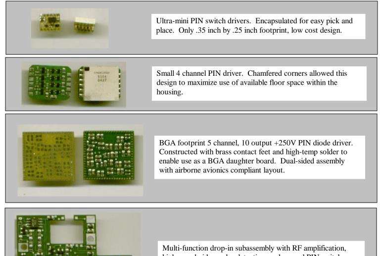
Multi-function drop-in subassembly with RF amplification, high-speed video pulse detection, and several PIN switch driver circuits in a user-friendly shaped layout. Backside is fully grounded for low loss and low-noise operation.
