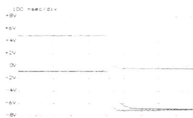
Voltage Settling Time, Shunt Uncompensated vs 20 pF/1k Comp
