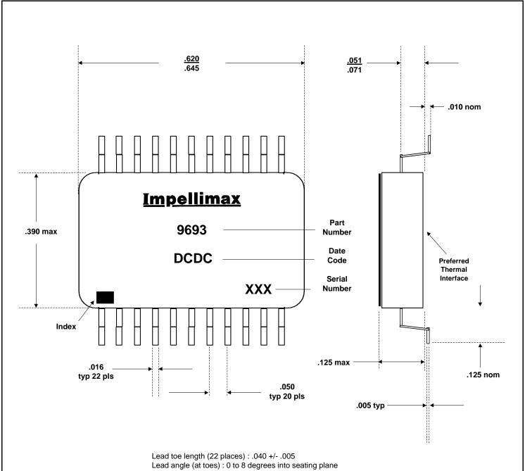
Lead coplanarity: .005 max Package Code 4
