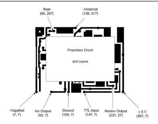
One Channel Moderate Speed Driver for GaAs MMIC Switching
