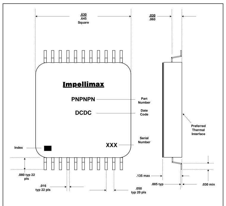
Leadforming is typically performed using EREM tool # 500-13A with #500-18 jaws.
